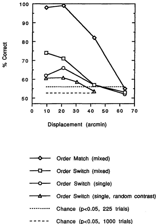
FIGURE 2. Results of Experiments 1 and 2, plotting mean per cent correct in a direction discrimination task as a function of displacement. Different curves represent results using different stimuli depicted in Fig. 1. Broken horizontal lines show the upper limit of chance responding according to cumulative binomial probability theory. For Experiment 1, chance = 56% ( $P < 0.05$ , 225 trials); for Experiment 2, chance = 52.7% ( $P < 0.05$ , 1000 trials).
